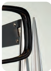
Non-parallel jaws can damage thick frames
